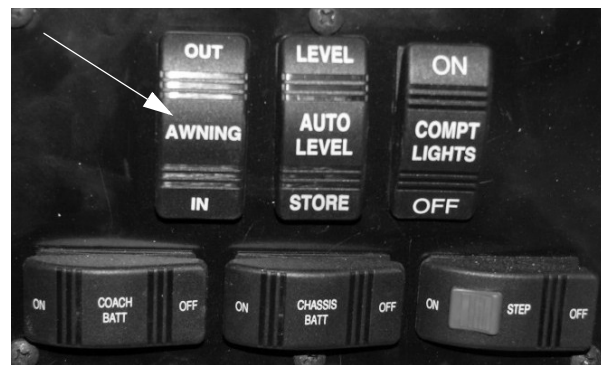
Patio Awning Control Switch (Located near entrance door) -Typical View
