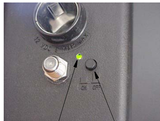
Power indicator glows when signal amplifier is active Push On-Off TV Signal Amplifier Power Switch (Located near entertainment center cabinet) -Typical View
