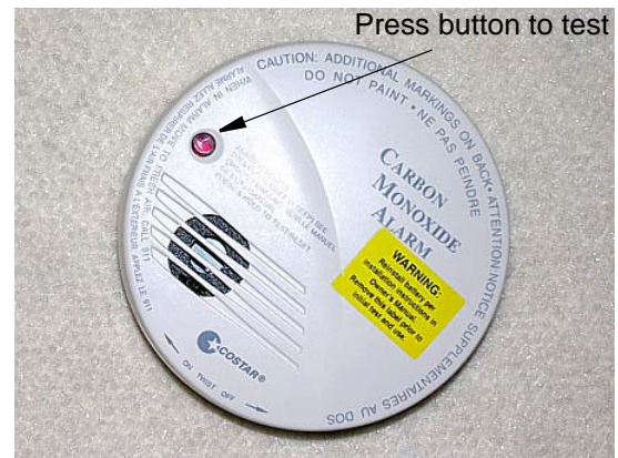
Carbon Monoxide Alarm
