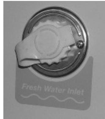
Fresh (City) Water Connection (Fresh Water Inlet)
