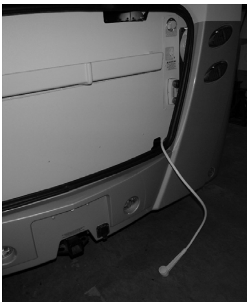
Using exterior shower to drain waterline
