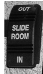
Slideout Switch (Your coach may have one or more slideout switches depending on model, options, and available equipment) -Typical View
