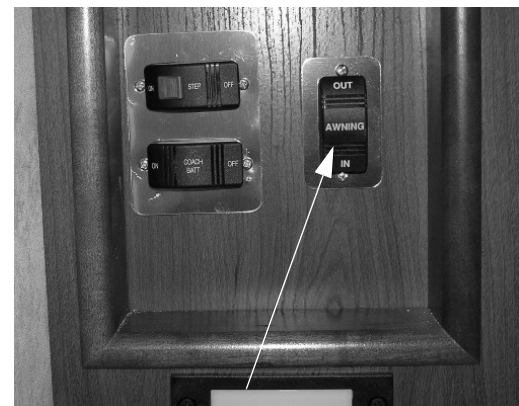
Awning Control Switch (Located near entrance door) –Typical View
