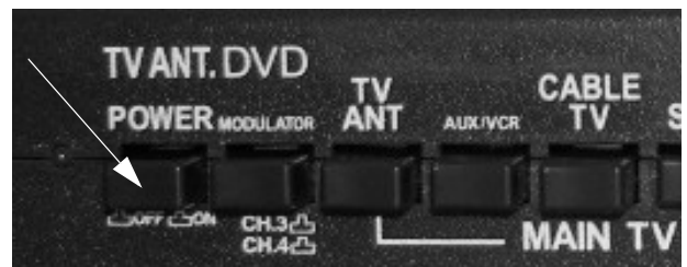
TV Signal Amplifier Switch (Located on Video Selection System)
