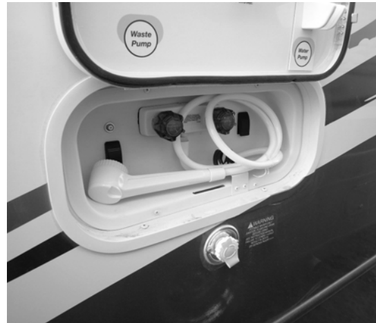
Exterior Shower/Wash Station -Typical View
