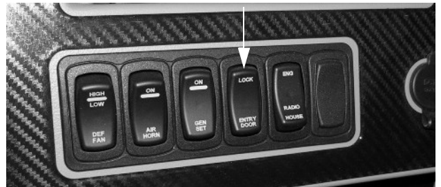
Power Door Locks - Entry Door (Located on dash) -Typical View
