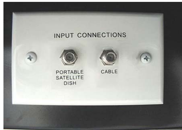
Exterior Connection for Satellite Dish and Cable TV (Located in utility compartment)
