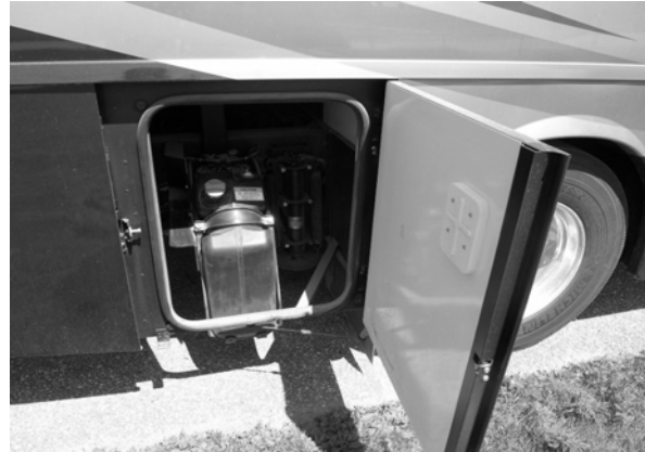
Diesel Exhaust Fluid Fill Tank (Located in passenger side compartment behind rear wheel) -Typical View
