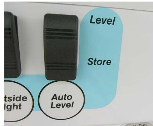
Auto Level Remote Switch (Located in utility compartment) -Typical View
