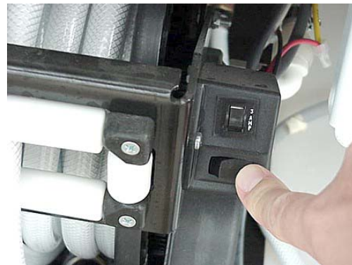
Press and Hold button to retract Water Hose Reel (If Equipped) -Typical View
