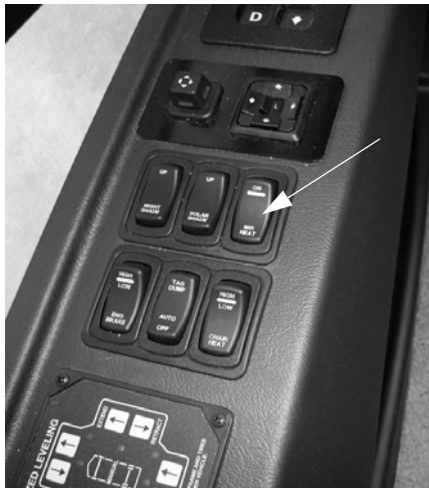
Mirror Heater Switch (Located on driver side trim panel) -Typical View
