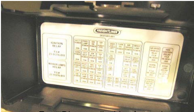
Fuse Diagram (inside of cover)
