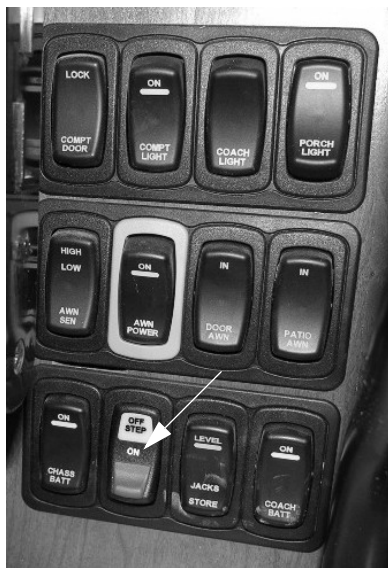
Entry Step Switch (Located near the entrance door) -Typical View
