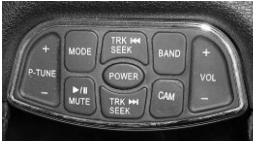
Steering Wheel Radio Remote Control
