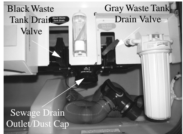
Black and Gray Waste Tank Drain Valves (Located in water service center)
