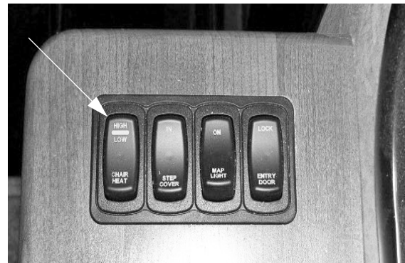
Chair Heat Control Switch (Located on driver and passenger side armrests) * Passenger side shown -Typical View
