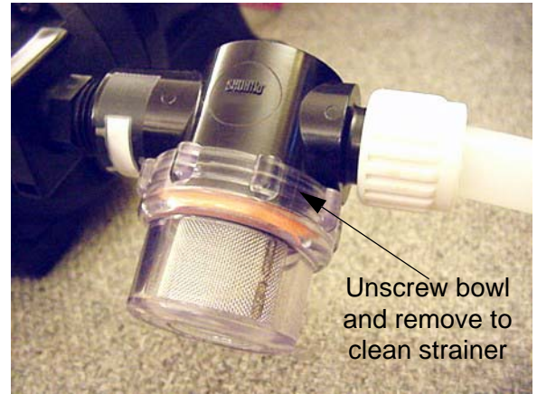
Water Pump Strainer -Typical View
