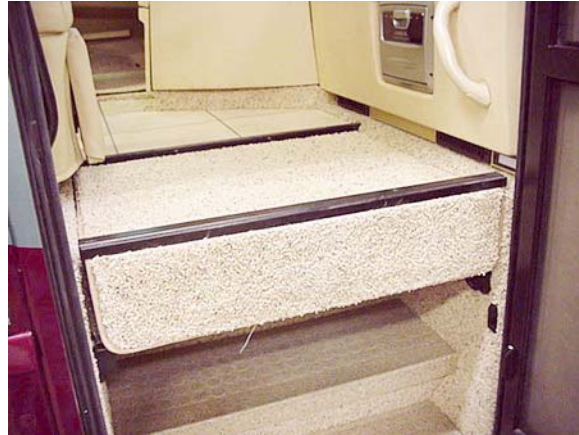
Stepwell Cover shown in extended position -Typical View
