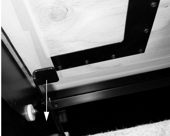
Emergency Retract Lever (Located underneath stepwell cover)
