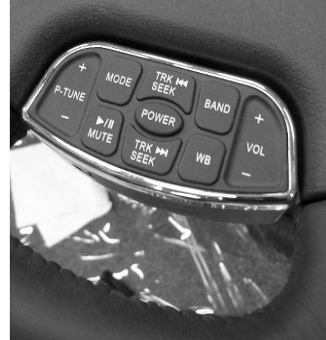
Steering Wheel Radio Remote Control
