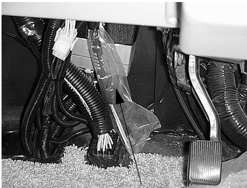
CB Power Wires (in plastic sheath) Typical View - your coach may differ
