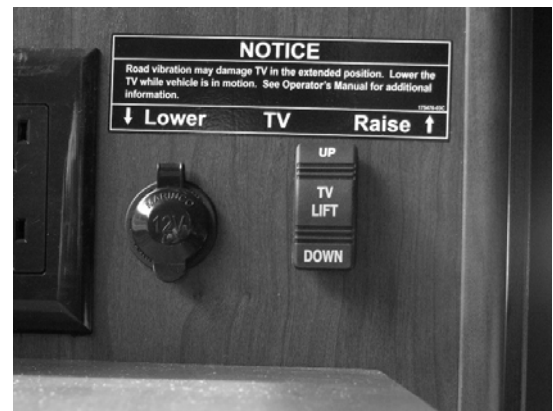
Power Lift/Lower Control Switch -Typical View
