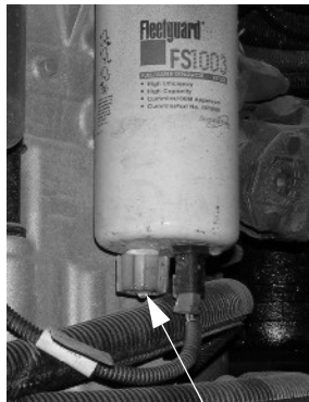
Fuel/Water Separator Drain Valve (Located on bottom end of separator) -Typical View
