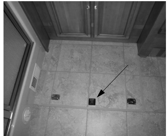
Rear Engine Access Cover Lock
