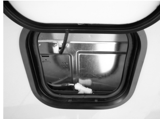
Residential Refrigerator Access Compartment -Typical View
