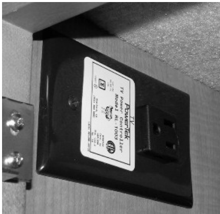
Front TV Ignition Switch Interlock -Typical View
