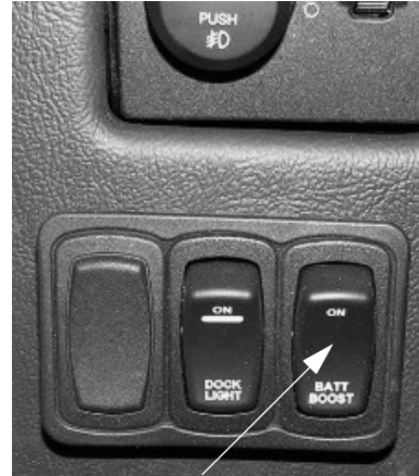
Battery Boost Switch (Located on dash)
