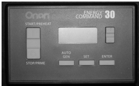
AGS Control Pad (Located near monitor panel)
