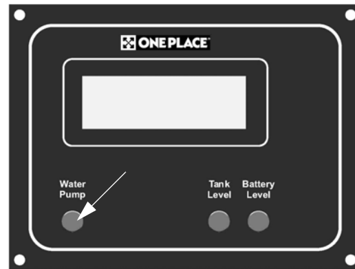
Water Pump Switch
