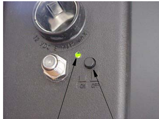
Power indicator glows when signal amplifier is active Push On-Off
