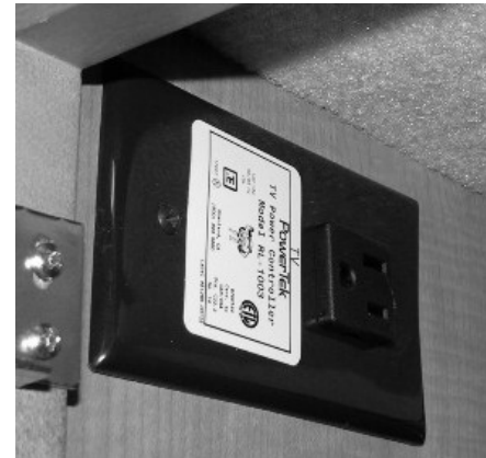
Front TV Ignition Switch Interlock -Typical View
