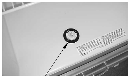
Place bubble level in bottom of refrigerator
