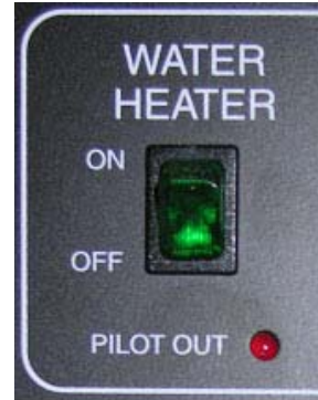
Gas Water Heater Switch (Located on Systems Monitor Panel)
