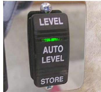
Auto Level Switch (Located near entrance door) -Typical View
