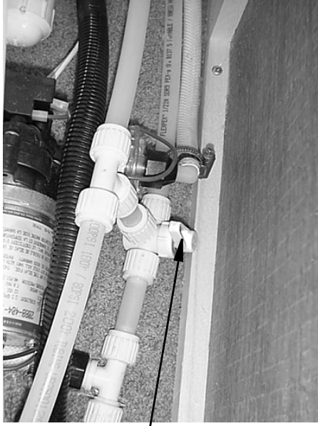
Waterline Drain Valve (Typical)
