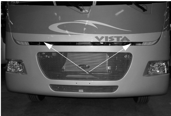
(Lift up the latches on each side of interior hood and raise)
