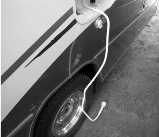
Using exterior shower to drain waterline (if equipped) -Typical View
