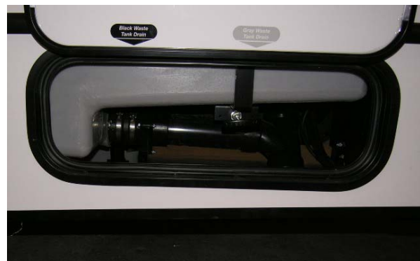
Holding Tank Dump Valves (Located in mid-driver side access compartment) -Typical View
