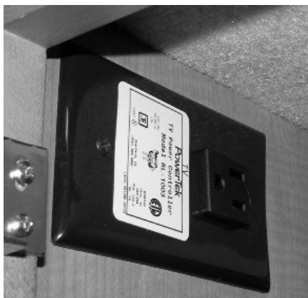
Front TV Ignition Switch Interlock -Typical View
