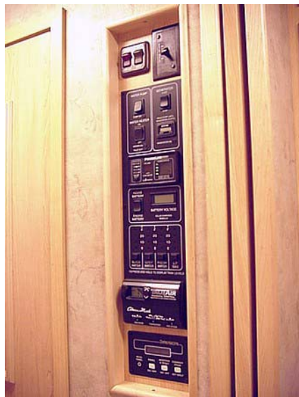
OnePlace Monitor Panel -Typical View
