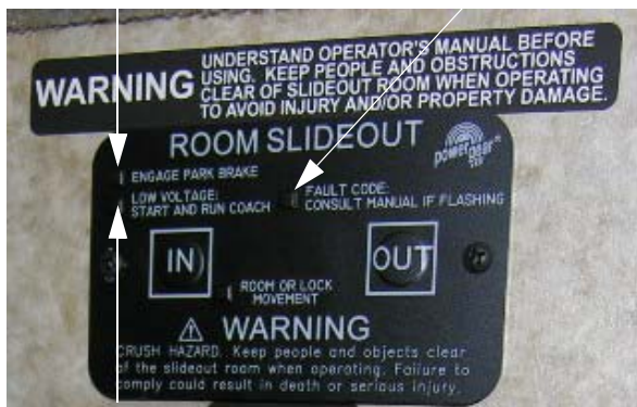
Low Voltage Indicator
