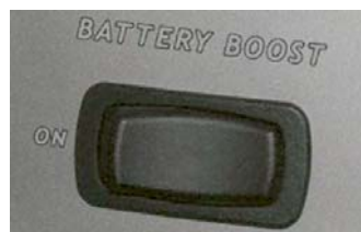
Battery Boost Switch
