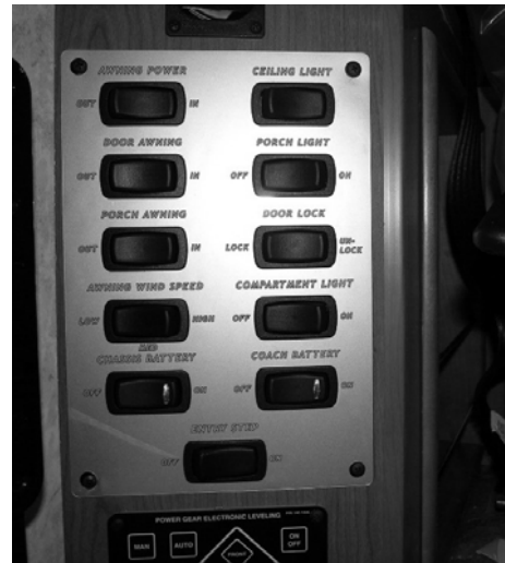
Awning Control Switches (Located near entrance door) -Typical View
