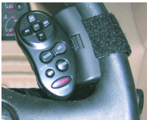
Radio Remote Control (Ford® Chassis) -Typical View
