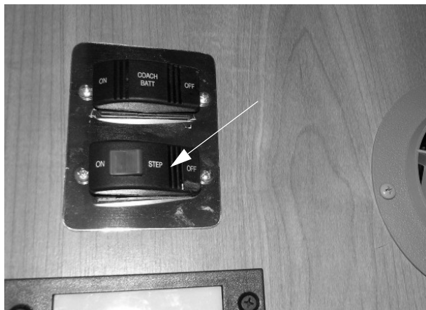
Entry Step Switch (Located near entrance door)
