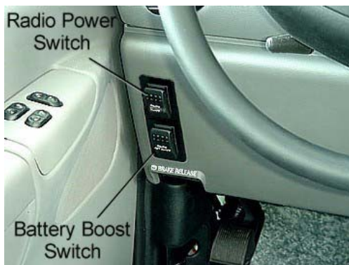
Battery Boost Switch
