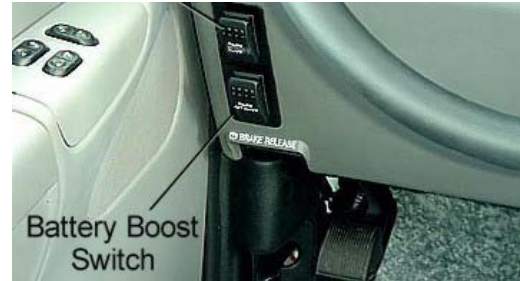
Battery Boost Switch
