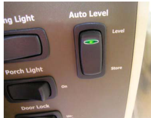
Auto Level Switch inside Entrance Door
