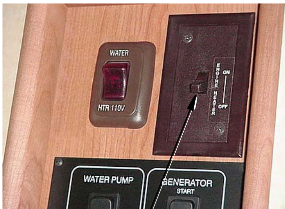
Diesel Engine Heater Switch (Typical)
