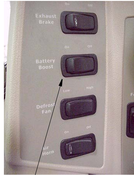
Battery Boost Switch
