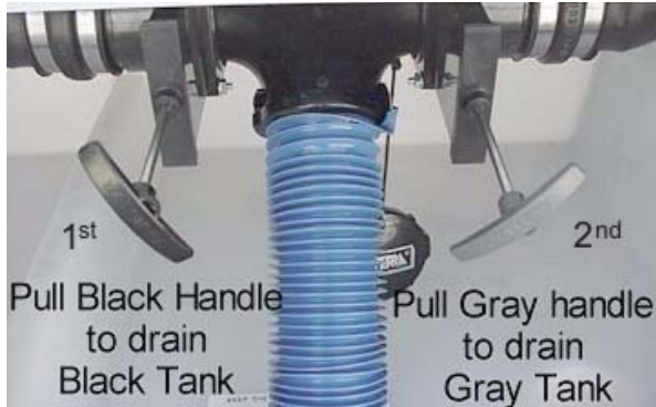
Holding Tank Valves (Typical)
