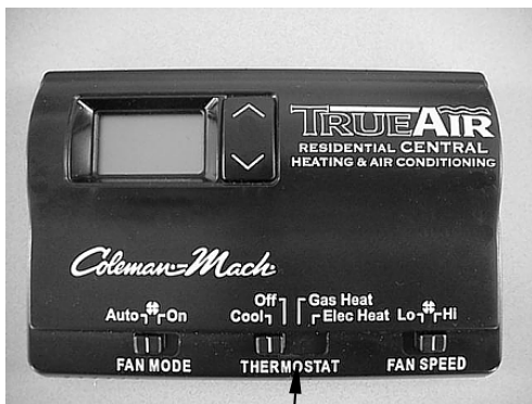
Thermostat Switch Gas Heat = Furnace Only Elec Heat = Heat Pump
