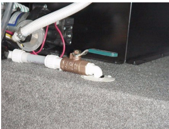
Water Line Drain Valve in RH Exterior Water Pump Compartment All Models
