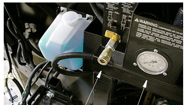
Quick-connect air coupler and air pressure gauge at front end of coach
