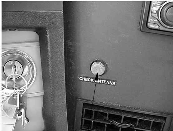
"Check Antenna" Light
