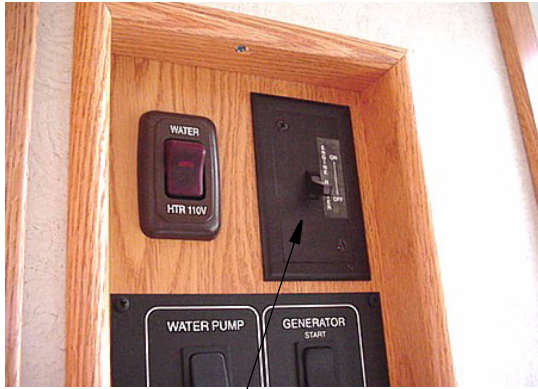
Diesel Engine Heater Switch
