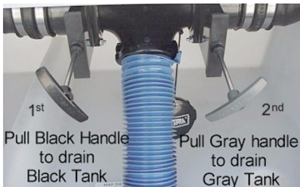
Holding Tank Valves (Typical)
