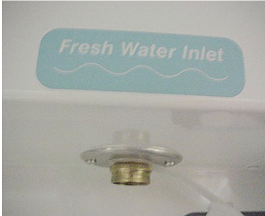
Fresh (City) Water Inlet
