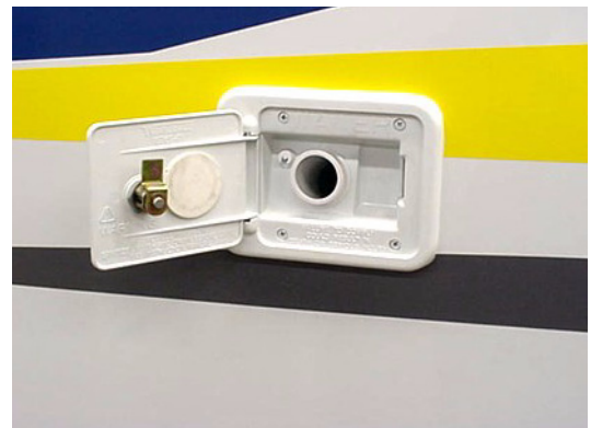
Water Tank Gravity Fill (typical)
